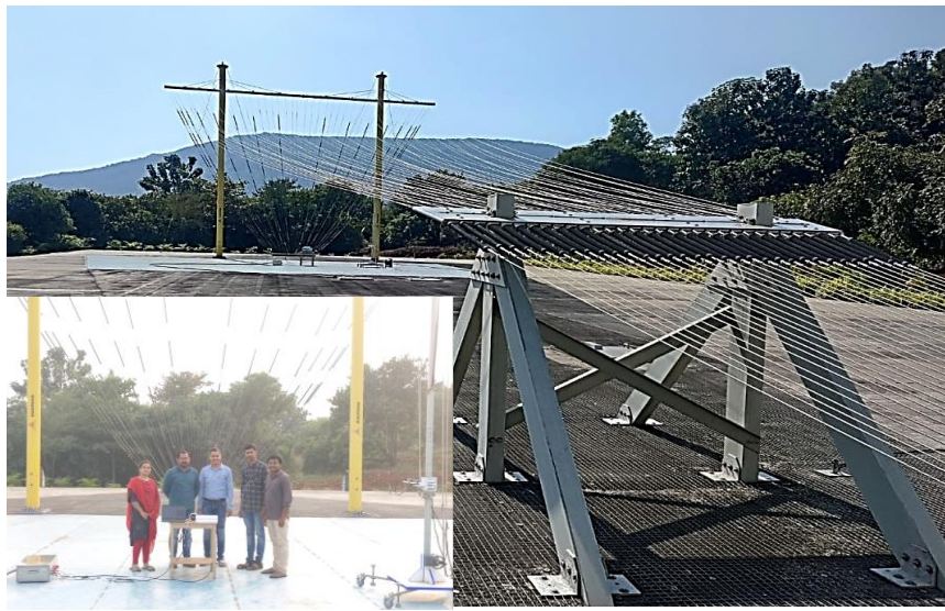
Pulsed Current Injection (PCI) facility for evaluating HEMP Filters for point of entry protection
