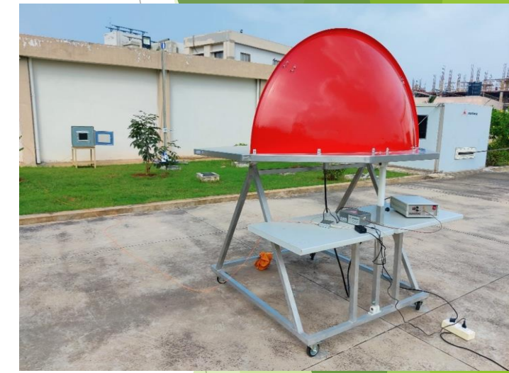
Facilities for evaluating the immunity against Lightning & Electrostatic Discharge
