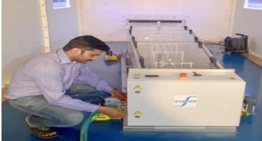
Pulsed Current Injection (PCI) facility for evaluating HEMP Filters for point of entry protection
