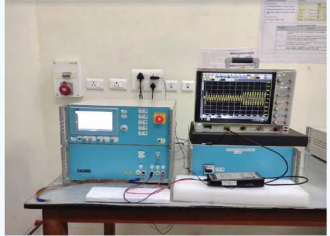
Voltage dips, short interruptions and variations Immunity test (IEC 61000-4-11)
