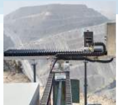
GB-SAR illuminating the OB dump benches Courtesy: NCL, Dudhichua
