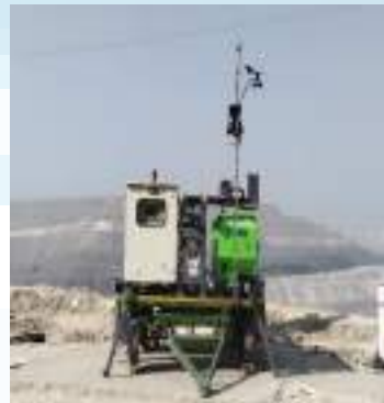
Ground Based- Slope Monitoring Interferometric SAR (GB-SMiSA Radar) Courtesy: NCL, Dudhichua
