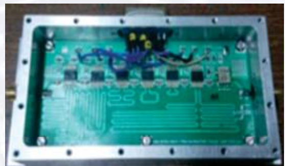
Six Bit Microstrip phase shifter developed for ST Radar
