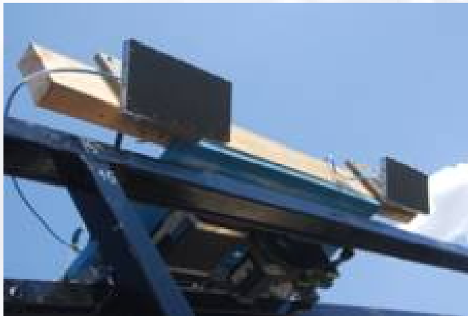
FMCW SAR experimental Set-up motorised rail
