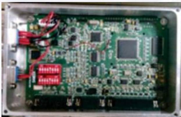
FPGA based TR module controller for ST Radar
