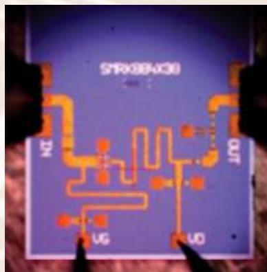
Simulation layout and fabricated chip of the U-band frequency tripler circuit
