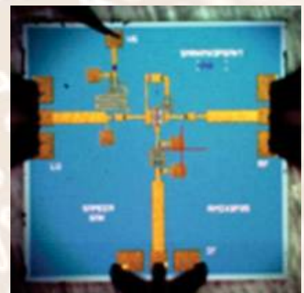
Fabricated two resistive Ka-band MMIC mixers
