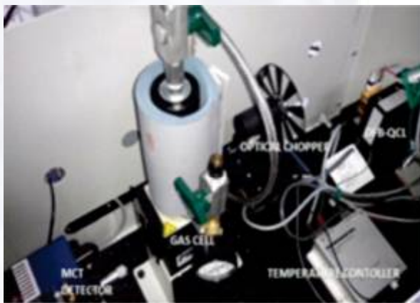
Lab Prototype for traces gas detection using multi pass gas cell
