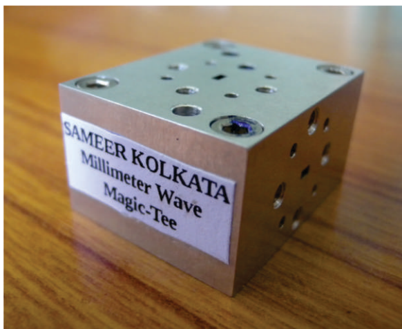
Millimeter-wave Magic Tee with measured S-parameters.
