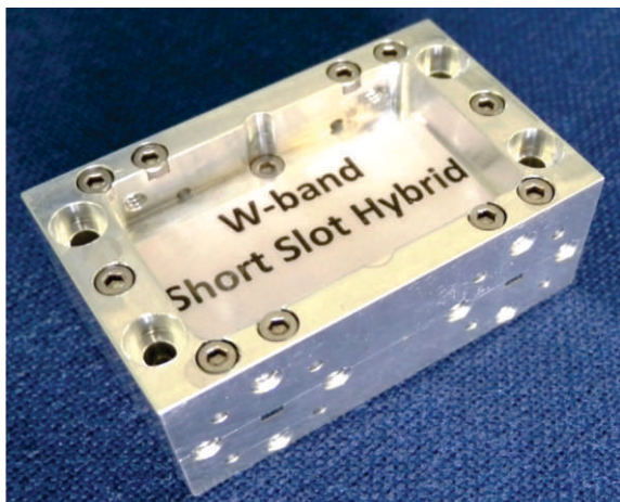
W-band Short slot hybrid with measured S-parameters.
