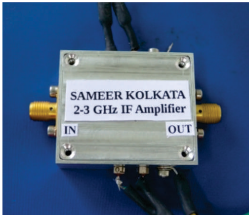
S-band IF Amplifier with measured output spectrum.
