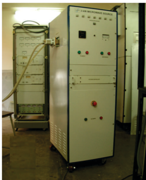
High Power Pulsed/CW Microwave System for processing of soy beans grain for Central Institute for Agricultural Engineering (CIAE)
