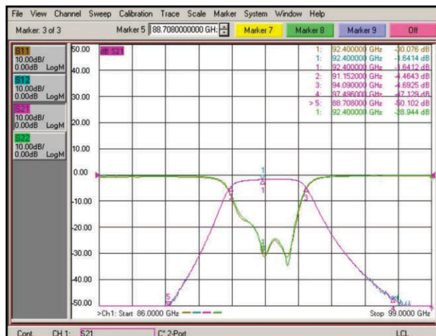
W-band low noise amplifier with measured S-parameters.
