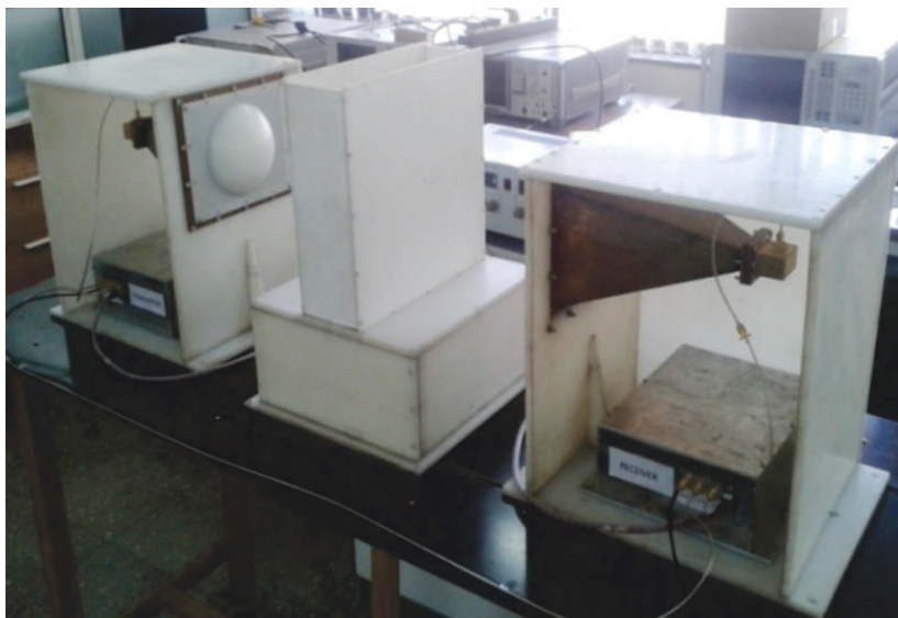
Measurement setup for moisture measurement
