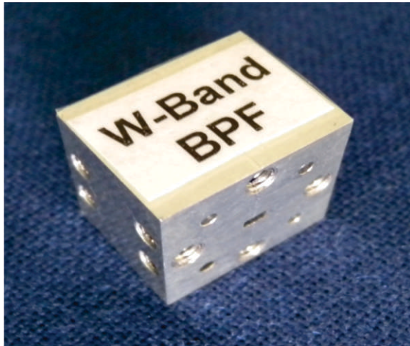
W-band narrow band pass filter with measured S-parameters.
