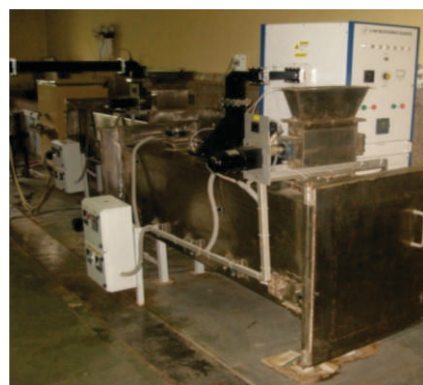
Variable Power Pulsed/CW Microwave System for processing of seeds for PUSA Institute
