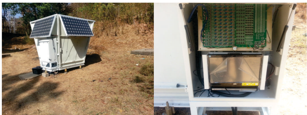
Phased Array SODAR System being tested at SAMEER campus
