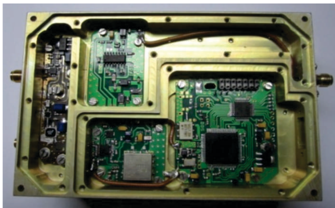
The RF module (DDS and PLO section)
