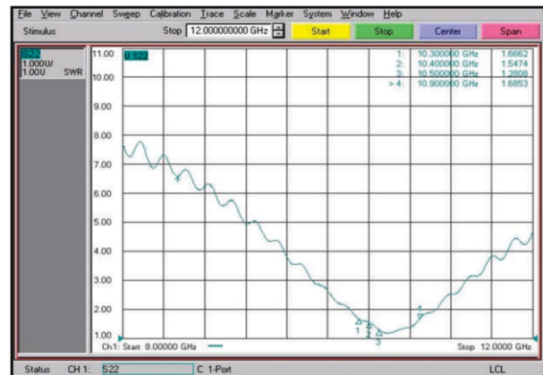
X-band data Link Receiving Antenna with measured VSWR
