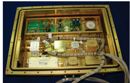
Developed unit of TR Module for ST Radar project.
