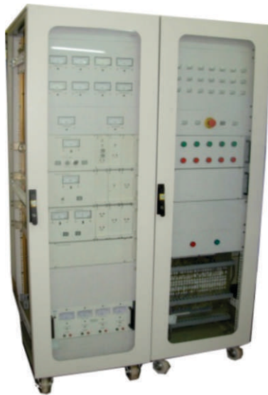
Low power controller rack of the 30 kW Transmitter at 75 MHz
