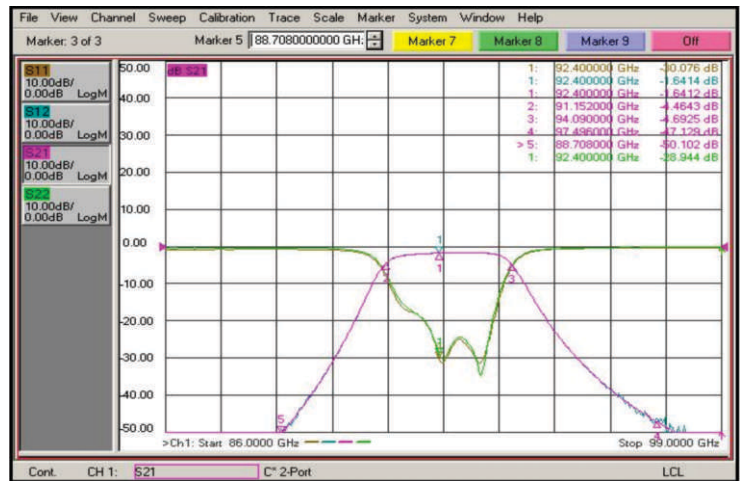
W-band narrow band pass filter with measured S-parameters.
