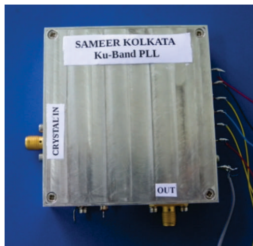
Phase Locked Oscillator at 14.25 GHz with measured output spectrum.
