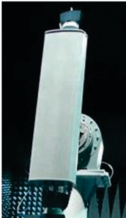
Base station antenna measurement
