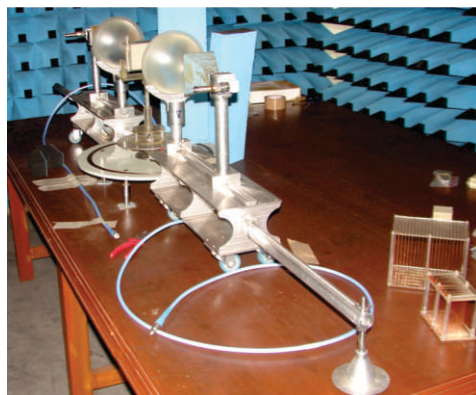
Mechanical set-up for characterization of left handed Maxell's system
