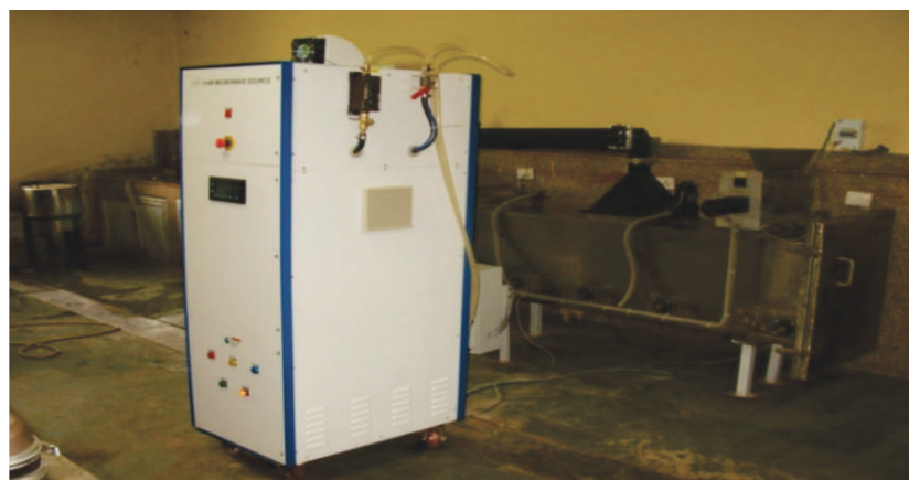
5 kW CW Microwave System for Drying Agro Products for Indian Agricultural Research Institute (IARI)
