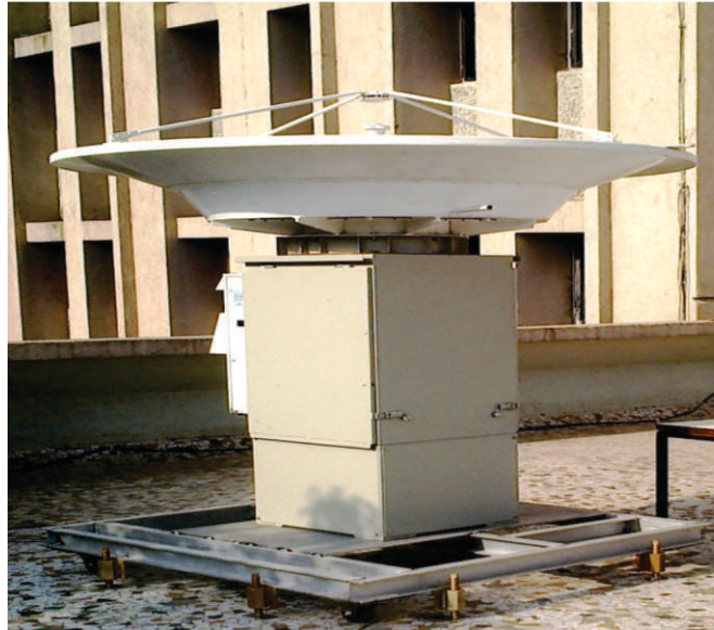
SAMEER's Ka-band zenith looking cloud profiling radar
