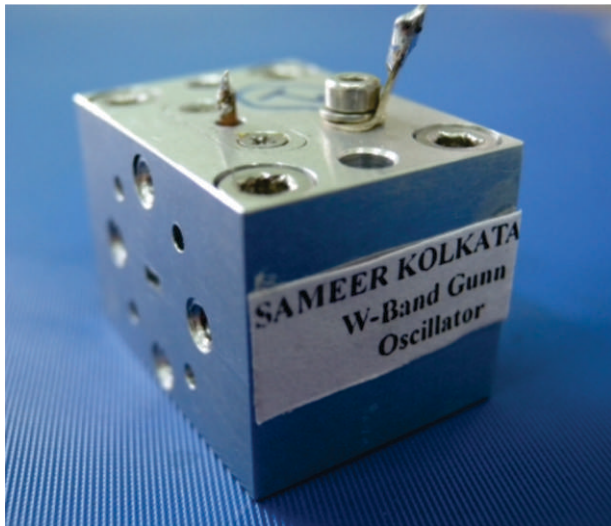
CW Gunn Oscillator Cavity with measured output spectrum.
