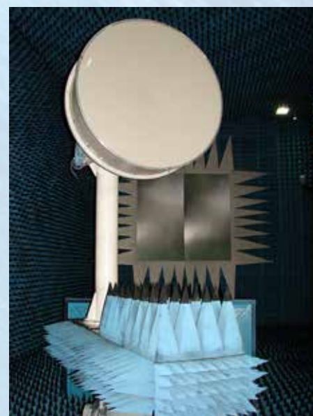
Photograph of the measurement set-up during radiation performance evaluation of a microwave communication antenna.
