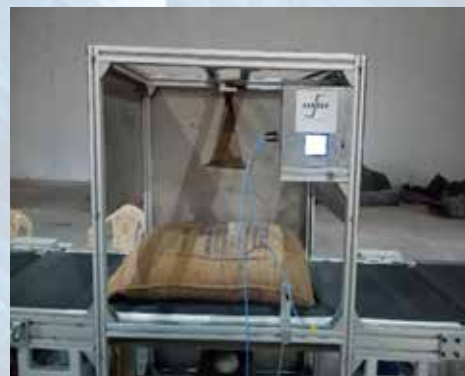
Online moisture meter mounted on the conveyer
