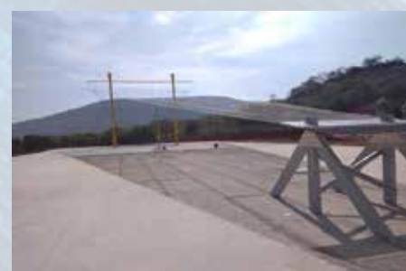
Photograph of the azimuth measurement set-up during radiation parameter measurement of the multiband wrap around antenna.
