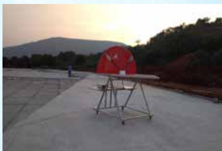
HEMP Pulse Current Injection (PCI) Test System As per MIL-STD-188-125/1&2 Installed at Site
