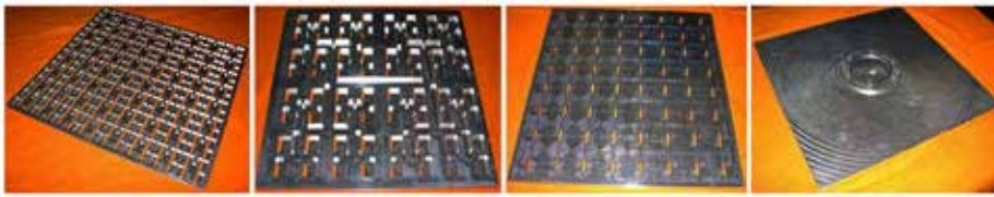
Different parts of the fabricated antenna. From left: top part (rear side), middle part (rear side), middle part (top side), and bottom part (rear side).
