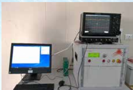
HEMP Pulse Current Injection (PCI) Test System As per MIL-STD-188-125/1&2 Installed at Site
