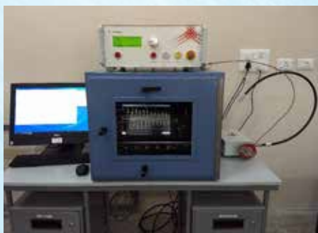
Ultra Wide Band (UWB) Test system Antenna, Generator and Measurement System Installed at Site
