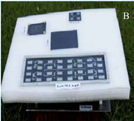
A prototype of the proposed SAA configuration with five antenna elements: (a) the top view (b) an isometric view
