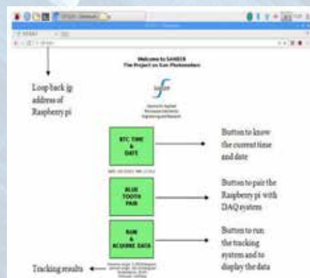
IOT feature of Auto Tracking unit
