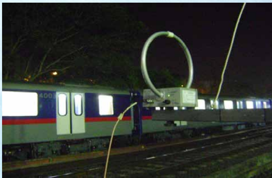
Radiated emission testing of Kolkata Metro rail
