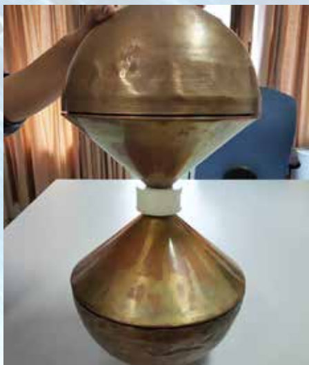
Structure of an Ultra Wide Band Spherical Dipole Antenna
