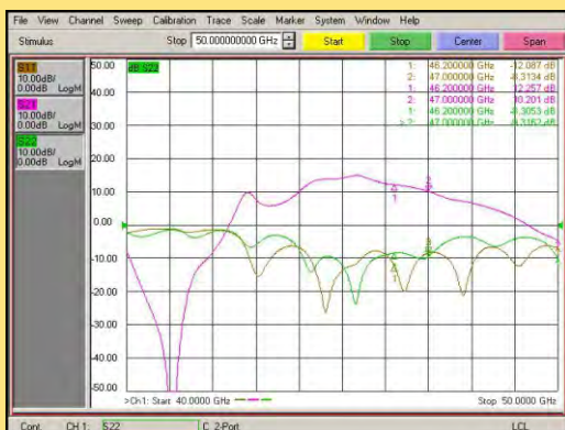
U-band medium power amplifier module and its measured frequency response
