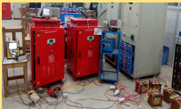
functional performance measurement of 10kw power conditioning unit of Statcon Power Controls Ltd., Noida at Customers premises. The performance of anti-islanding operation was also evaluated.
