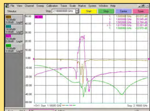
3-channel IF section at 1.6GHz and its measured frequency response
