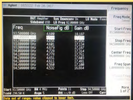
w-band LNA, measured gain and reflection coefficients and its Noise Figure
