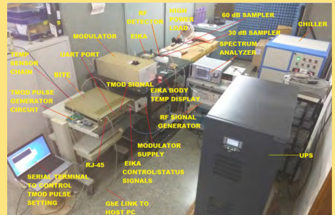
Testing of EIKA using our own make Controller & Monitoring Unit (CMP)
