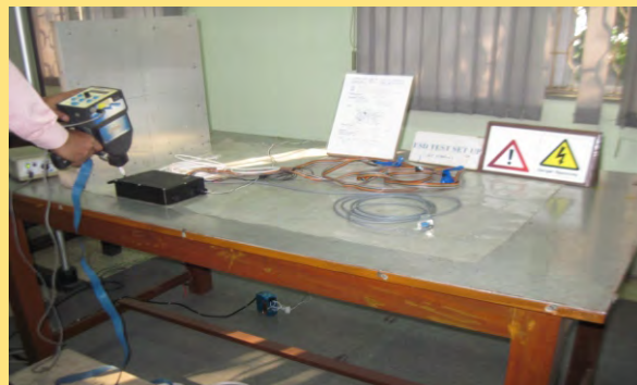
ESD test set-up for Site Monitor of M/s. AQ ElteknikABAlsikegatan, Uppsala, Sweden.
