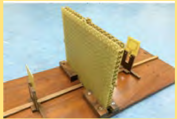
Metamaterial based flat lens at 65MHz (Unit cell size /500)
